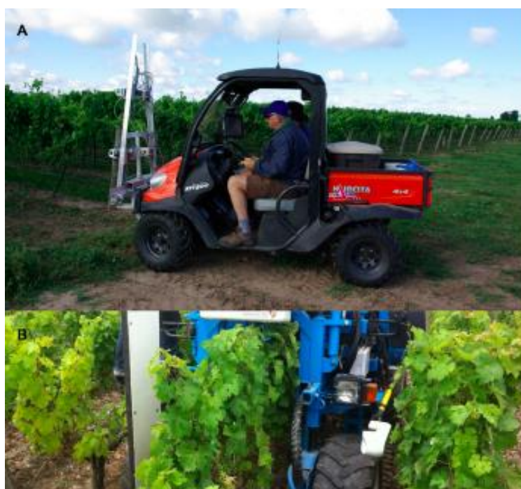
Figure 4. The Trimble GreenSeeker multispectral sensor for canopy monitoring, carried on a quad (practical Precision Inc., Tavistock, Canada) (A) or tractor (Avidorhightech SA, Le Mont-Pelerin, Switzerland) (B).
