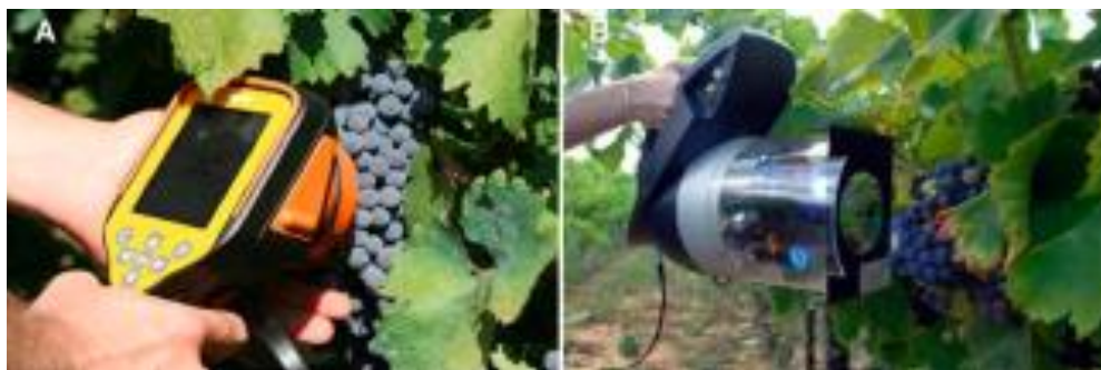
Figure 6. Spectron (A) and Multiplex (B) hand-device sensors for grape quality proximal monitoring, which allows quality maps to be realized
